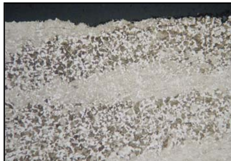
Failure Analysis gear and pinion shaft from excavator identifying extreme chemical segregation through microstructure analysis.
