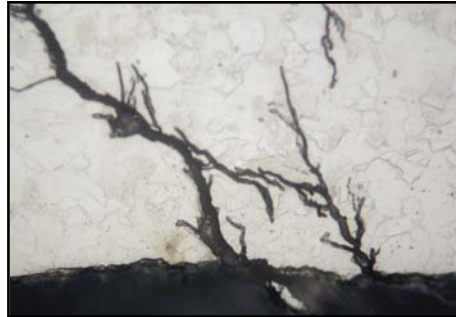
Failure Analysis of Ethanol plant stainless steel process tubing identifying stress corrosion cracking from exposure to unauthorized CIP materials.
